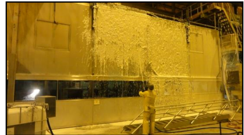
(Paper Machine Drying Section hoods Being Eco Washed)
